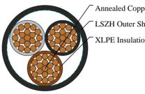
Annealed Copper Conductor LSZH Outer Sheath XLPE Insulation
